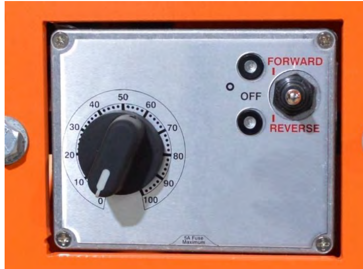
Pump Control Panel
